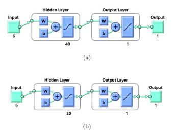
**Fig. 4** Designed ANNs architecture for yield prediction in (a) Trans Nzoia and (b) Nakuru counties.
