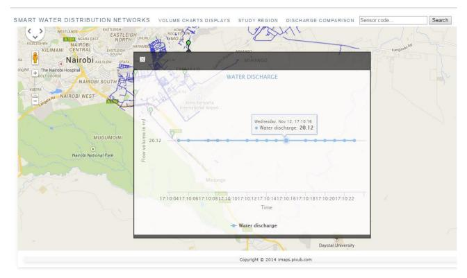
Figure 11 Sensor water discharge graph visualization
