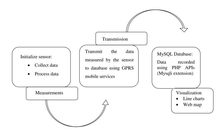
**Figure 6 Simplified implementation flow diagram**
