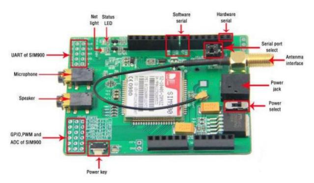
Figure 4 A SIM900 GSM shield.
